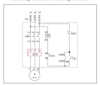
d.Connection diagram of YCQJ7 in case the main circuit voltage is AC380V and the control circuit voltage is AC220V
