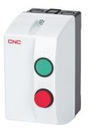
YCQ7 series magnetic starter is suitable for using in the circuits the rated voltage up to 660V, AC 50Hz or 60Hz, rated control power to 45kW and current to 95A. It is used to control the direct start and stop of the motor, and the starter with thermal overload relay protects the motor from overload and phase failure. Standard: IEC/EN 60947-4-1.
