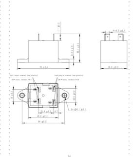
2、YCC8DC-60~100 Product appearance, installation, and wiring diagram
