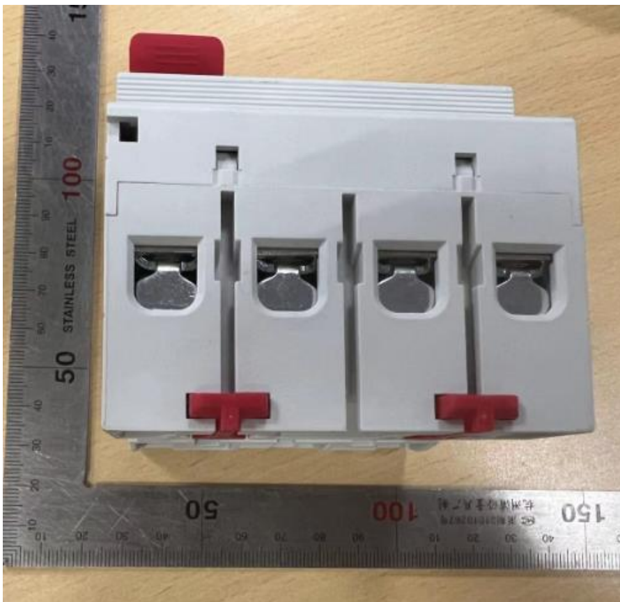
Sample of photo documentation (3P+N, 6A, type AC, 300mA)
