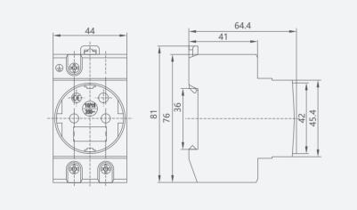
The socket must be installed and connected by professional electrical personnel. The socket is mounted on DIN 35mm guide rail, the tightening torque is 2.5 N.m.
