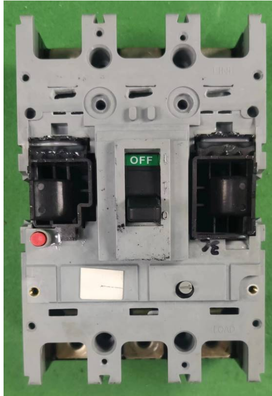
Internal view without front cover, YCM7T/A-250M/3300, 3P 100 A
