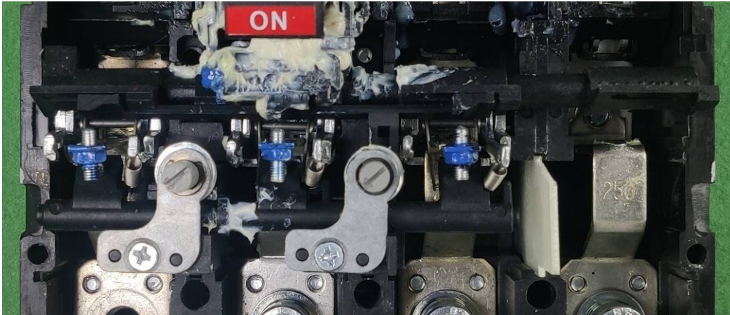
View of thermal bimetal components and leading lever, 55 °C YCM7RT-250M/4300, 4P, 250 A
